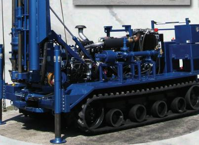
The D-120 is a large, heavy-duty, high power, multi-purpose drill rig. This drill has earned a reputation as a powerhouse in the geotechnical, exploration and environmental drilling industries. The D-120 is powerful enough to handle large diameter hollow stem augers, yet versatile enough to drill efficiently on small auger, rotary and core jobs. If you need more power, more capacity and more productivity, the D-120 is the drill for you!
